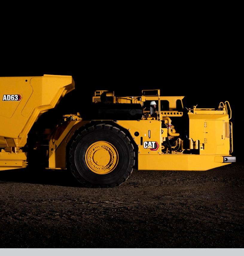
The new 63 tonne (69 tons) AD63 underground articulated truck is powered by the Cat® C27 engine that meets EU Stage V Emission Standards.
