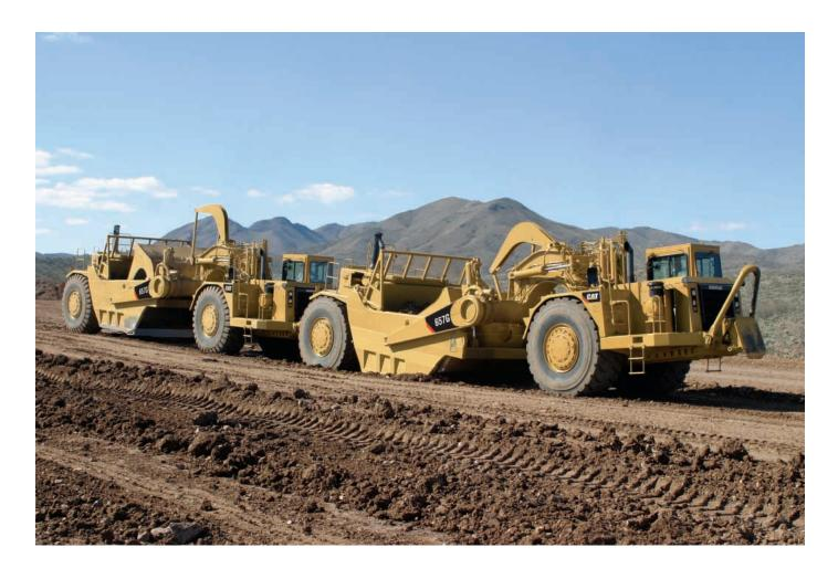
**Push-Pull Attachment.** This optional arrangement concentrates the combined horsepower of two machines onto one cutting edge. The push-pull attachment allows two individual machines to act as a self-loading system, typically loading both machines in less than a minute.
